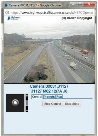
A virtual joystick in the bottom left controls the pan and tilt movement of the camera. The further away the joystick is dragged from the centre, the faster the camera will move. Next to the joystick is a zoom control. Moving the bar up and down controls the zoom in and out functionality of the camera respectively.
